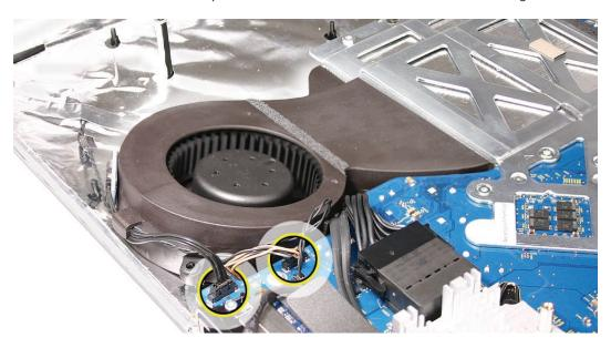
2. Lift the CPU fan from the system. Disconnect the ambient temperature sensor cable from the sensor.
